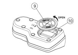
9. Battery Cover 10.Battery Compartment
